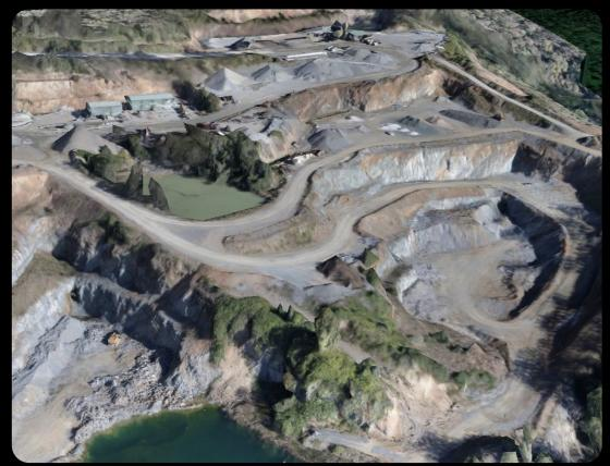
Digital elevation models (DEM) are visual representations of elevation data for every point captured on your site.
